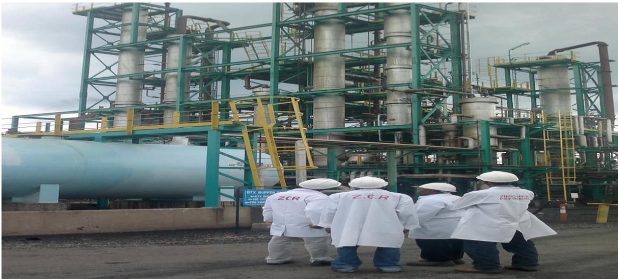
Beneficiation and value addition of products from coal: refining of by-products from conversion of coal to coke involves refining crude benzole to benzene, toluene & xylene and refining crude tar to creosote, road tar and soft pitch
